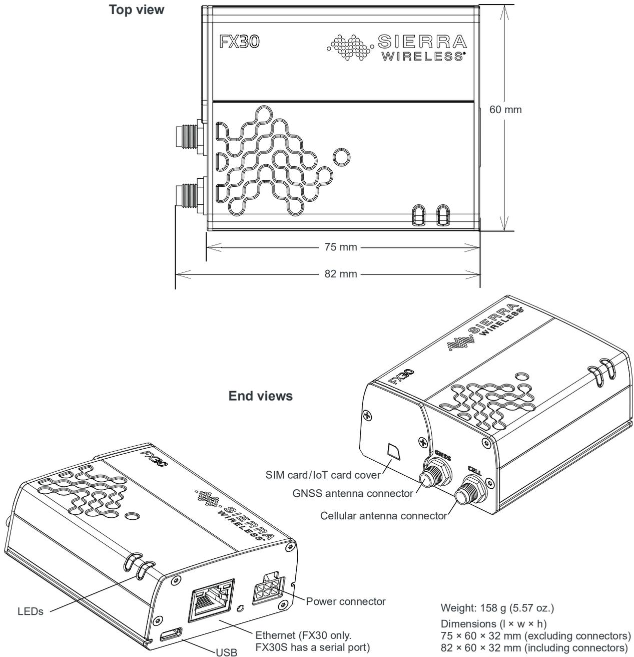
Figure 3-3: Mechanical Specifications
