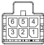
Figure 2-14: FX30S Power Connector
