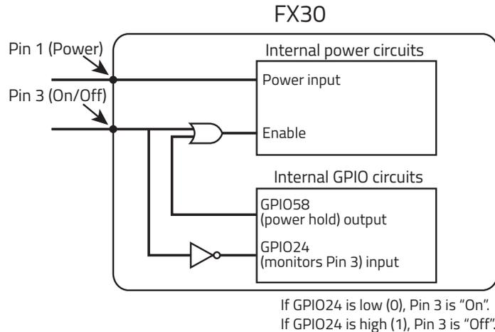
Figure 3-6: FX30S On/Off functionality
