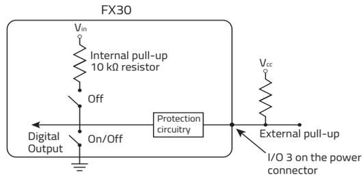
Figure 2-24: Digital Output/Open Drain
