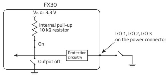
Figure 2-20: High Side Pull-up / Dry Contact Switch Input
