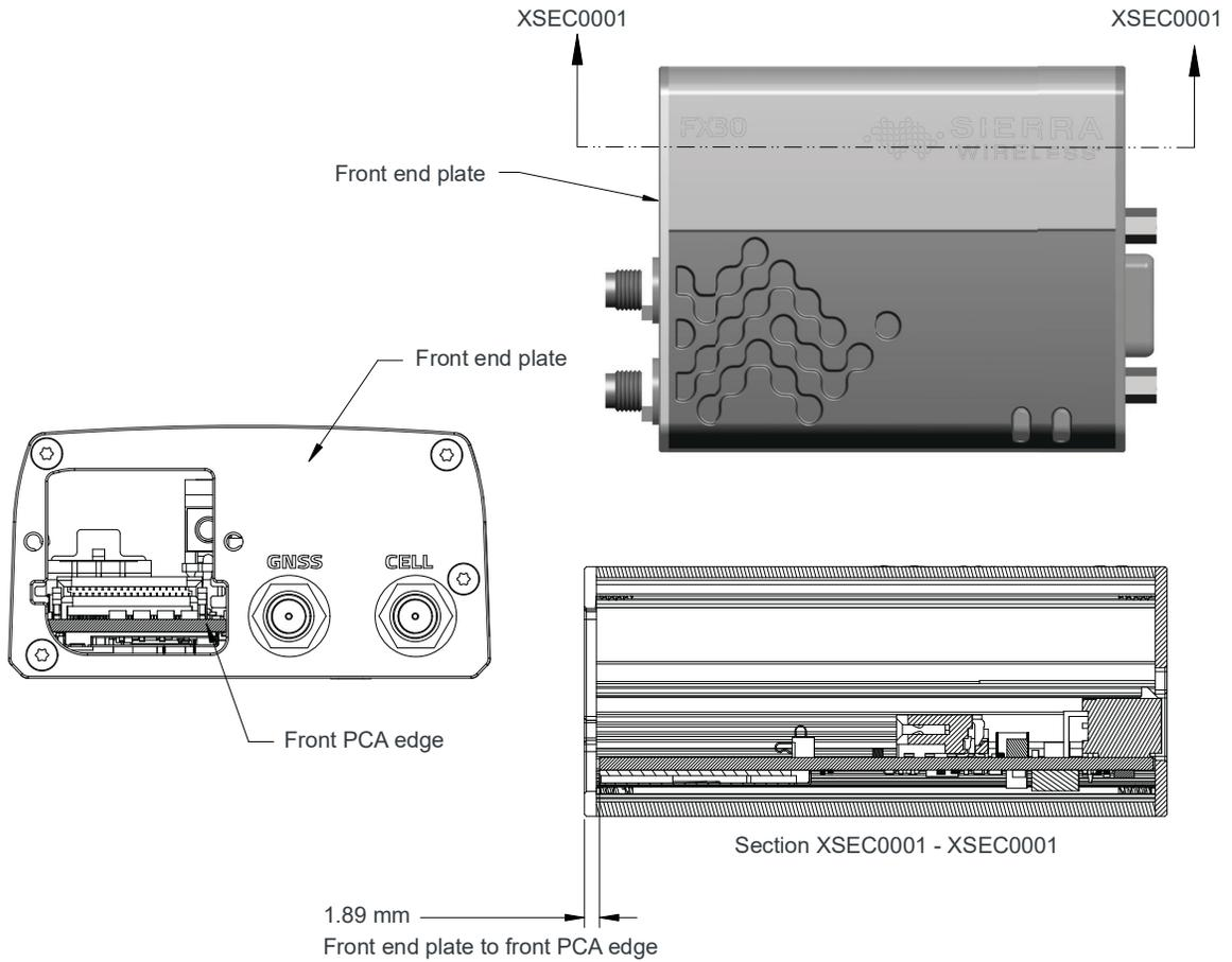
Figure 3-7: IoT Expansion Card Alignment
