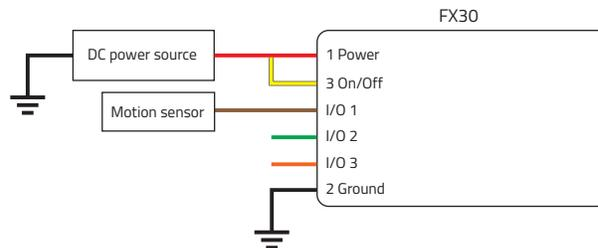
Figure 2-18: Fixed Installation with I/O
