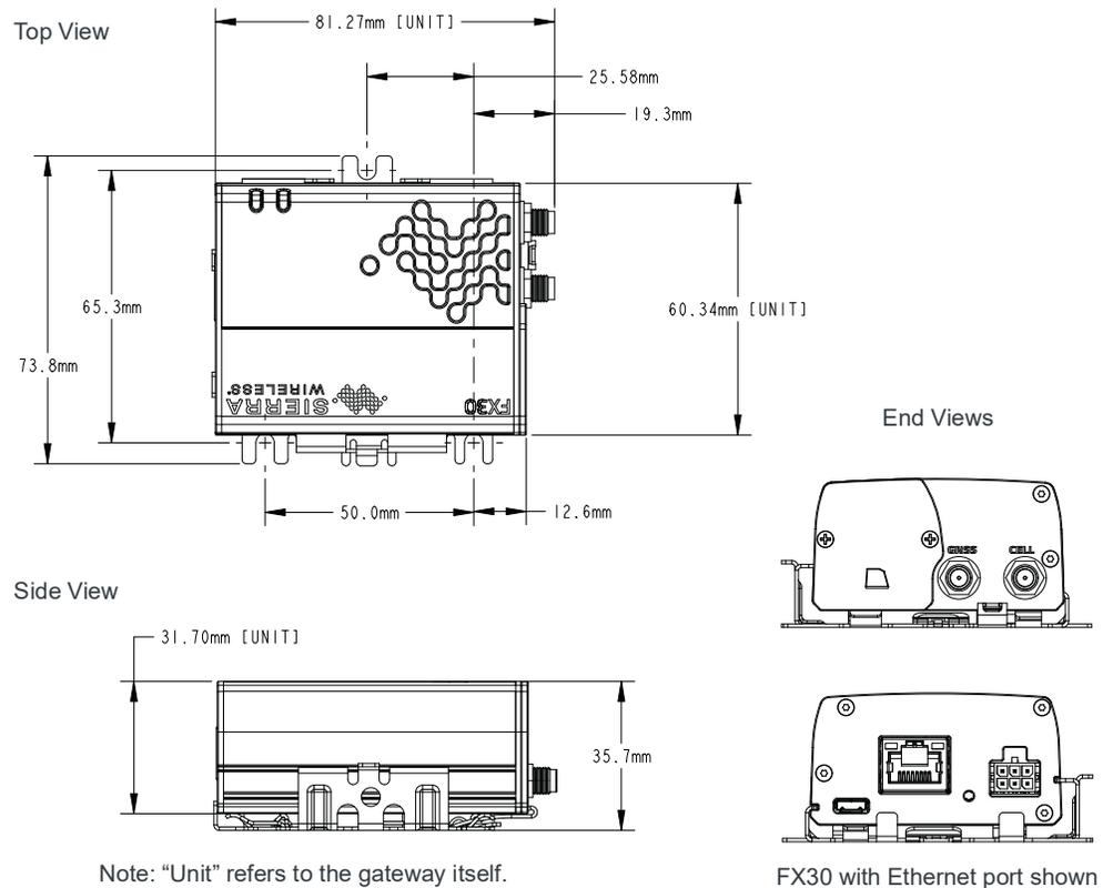
Figure 3-5: On mounting bracket
