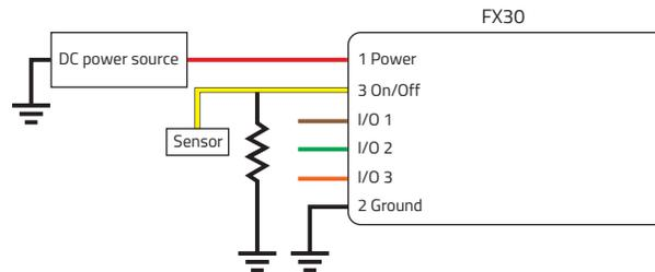
Figure 2-17: On/Off Installation (with sensor)
